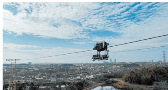
“Overhead power transmission line imaging inspection system” that automatically detects abnormal section through deep learning
