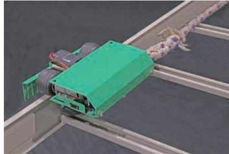
Device laying extension wire rope for cabling:
