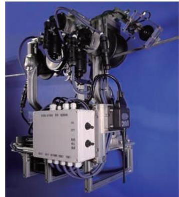
Self-propelled robot for removal of snow resistant rings
