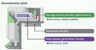
Incorporating NAS® batteries and solar power systems to amass knowledge about storage battery usage (Kinden Osaka head office)
