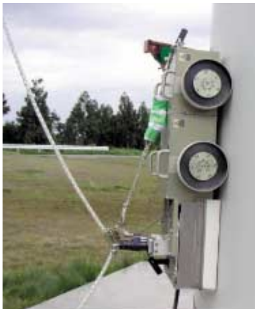
Close-up view of the self-propelled renovation painting robot
