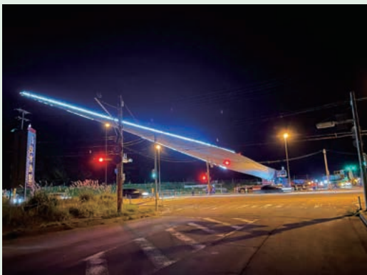
Standing up the blade and enabling it to rotate
